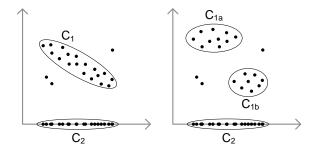
Figure 2: Local and global redundant clusters
